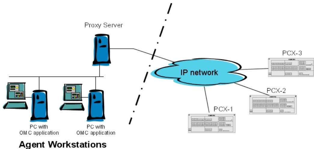
Figure 6.21: Configuration Example with a Proxy Server
