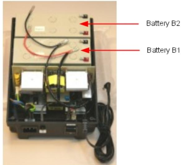
3. Connect the negative (black) terminals of the batteries as described below (and shown in the figure below).
