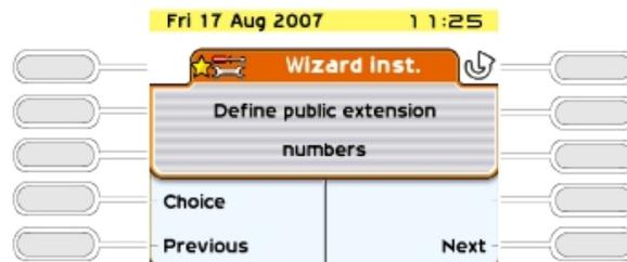
Access to the definition of terminal DDI numbers; displaying the first internal directory number/DDI number.
