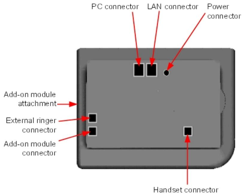
Figure 4.41: Alcatel-Lucent IP Touch 4028 Phone, Alcatel-Lucent IP Touch 4038 Phone and Alcatel-Lucent IP Touch 4068 Phone connectors
