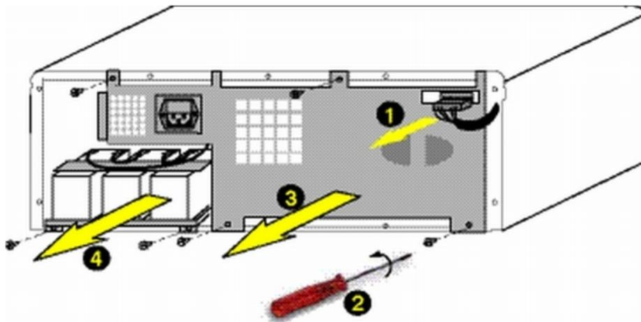
5. Replace the battery cable with the new cable provided with the connection kit (3EH 75031 AA).
