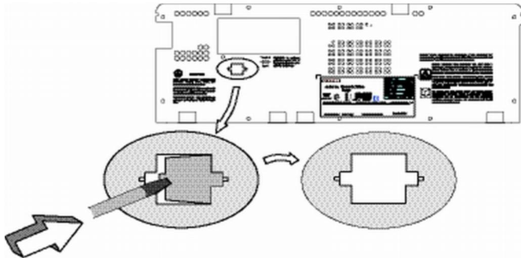
4. Remove the fan connector, then remove the power supply unit and the battery unit.
