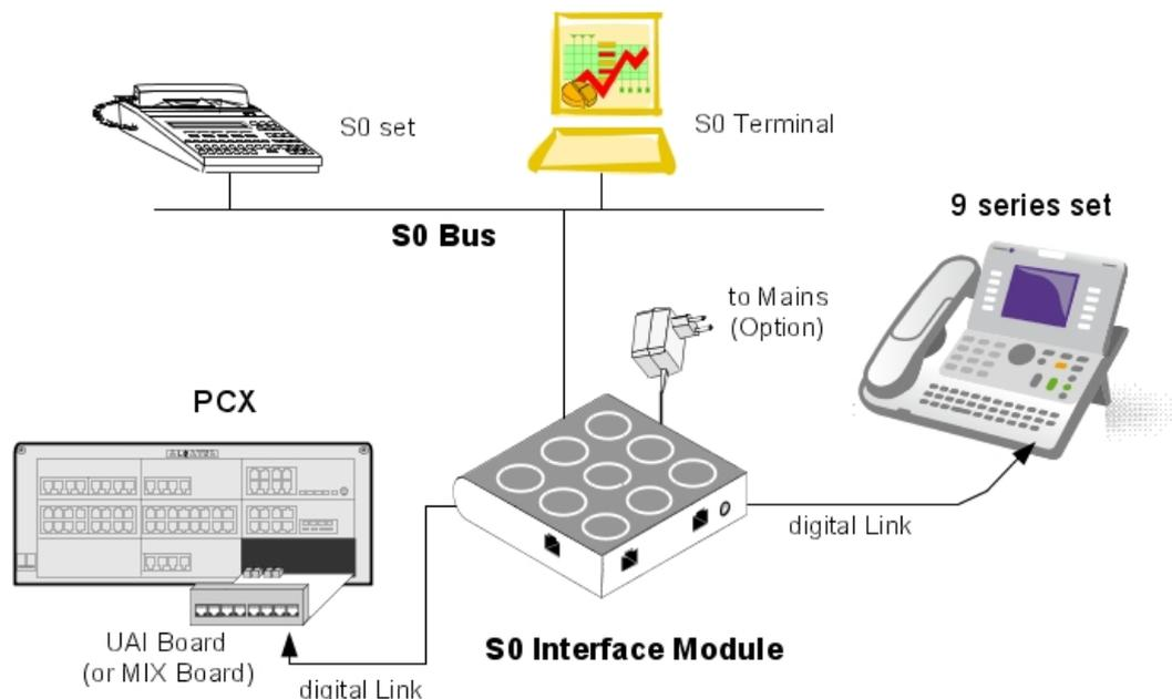
Figure 4.56: Example of Configuration with an S0 Interface Module
