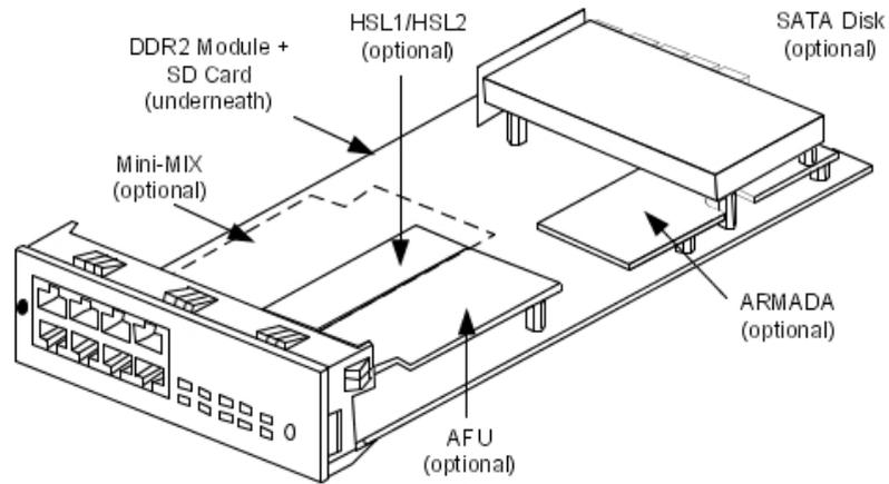
Figure 2.22: Example of GPU with SATA Hard Disk [Daughter Boards on PowerCPU](#)
