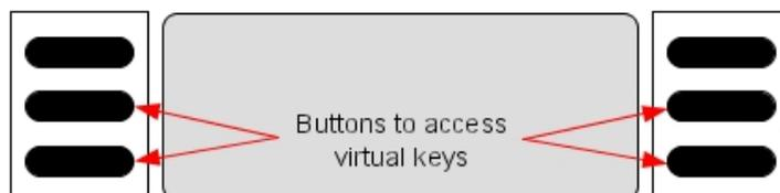
There are 10 pages of virtual keys (the pages can be scrolled through using the up/down buttons of the set's 4-way navigator), with 4 virtual keys on each page.
