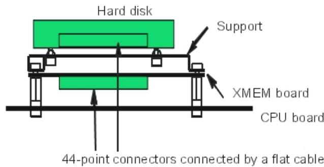
Figure 4.81: PATA Hard Disk Connection
