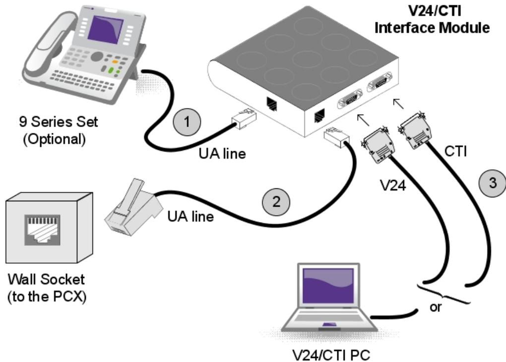
Figure 4.47: V24/CTI Interface Module Connection
