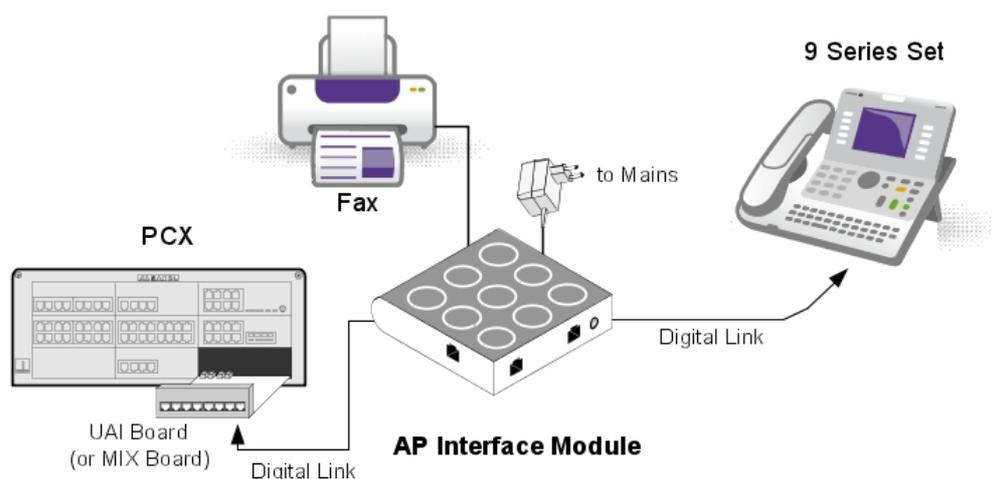
Figure 4.50: Example of Configuration with an AP Interface Module
