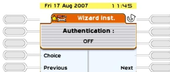
This is used to make secure data transmission between the system and DECT mobiles by using an authentication code during registration
