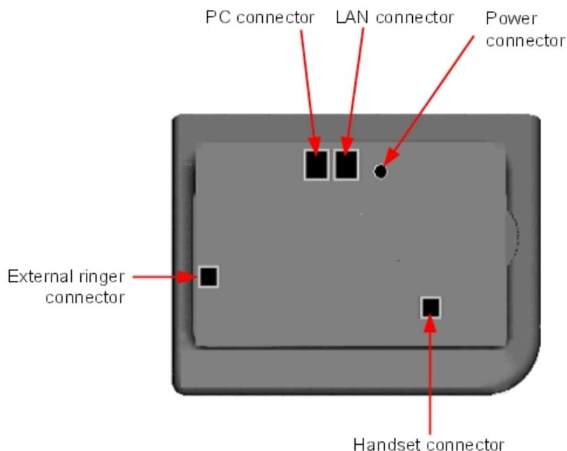
Figure 4.40: Alcatel-Lucent IP Touch 4018 Phone and Alcatel-Lucent IP Touch 4018 phone Extended Edition connectors
