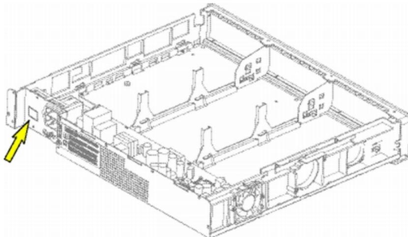
6. Connect the cable provided with the installation kit, and plug the connector into the rear panel and the slot. Secure the ferrite using the bracket and the self-adhesive base in the battery housing.
