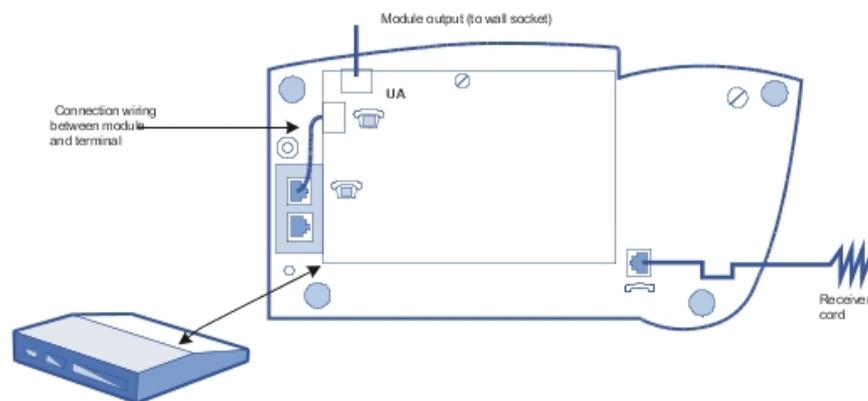
Example of using optional modules: connecting a charge management system
