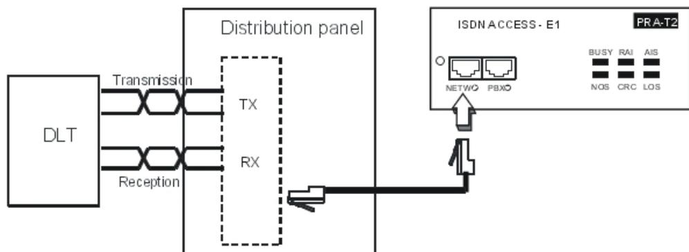
The PRA board is connected to a digital line termination (DLT) by 2 symmetrical twisted pairs.
