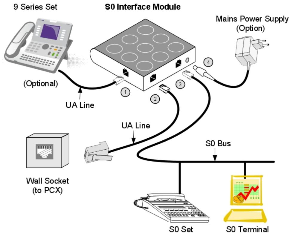
Figure 4.59: S0 Interface Module Connection
