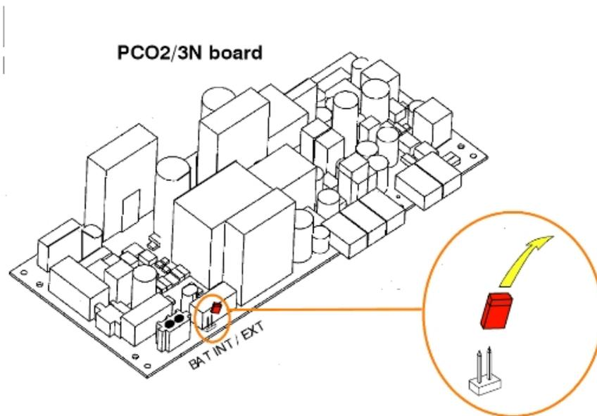
7. Remove the mounting clip and the batteries from the internal battery support.
