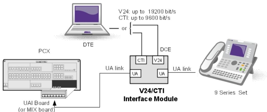
Figure 4.44: V24/CTI Interface Module Configuration Example
