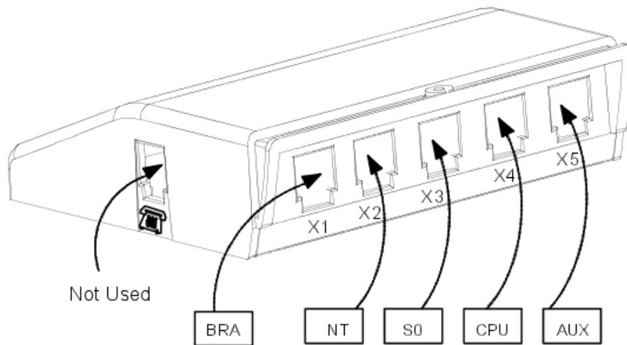
The ISDN-EFM box must be installed as close as possible to the system (3 m maximum). All the box connections are made with straight RJ45-RJ45 cables.
