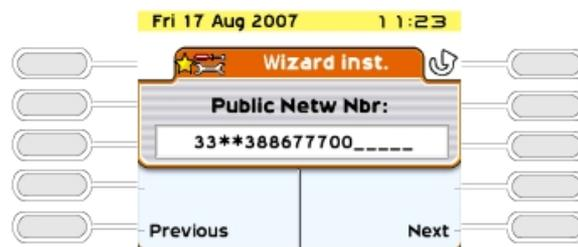
**This number must be entered in its entirety.** The number of your installation can include a maximum of three fields for a total of 18 digits.
