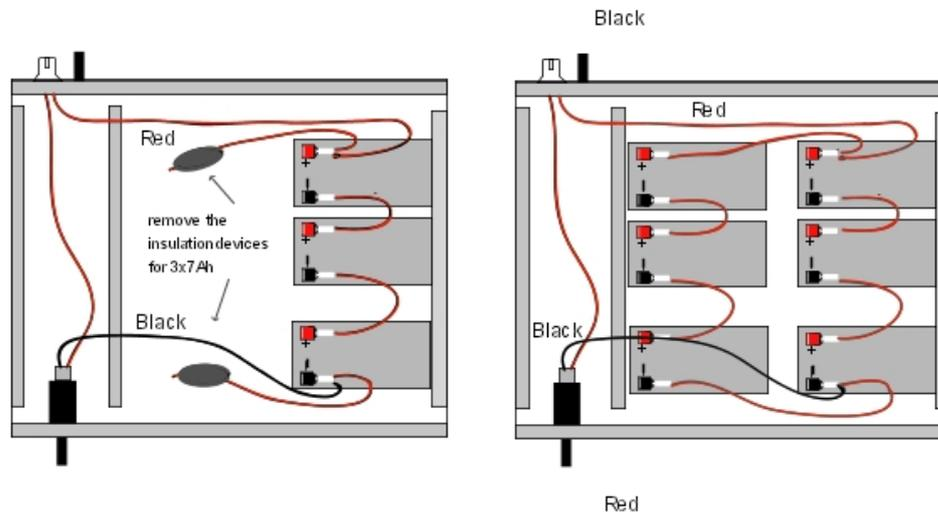
Figure 4.25: **Wiring Diagram of a 36V External Battery Rack Unit (1 or 2x7Ah in parallel)**
