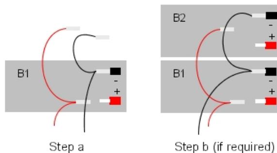
4. Connect the positive (red) terminals of the batteries as described below (and shown in the figure below). Note that there may be a small amount of electrical arcing when electrical contact is made.
