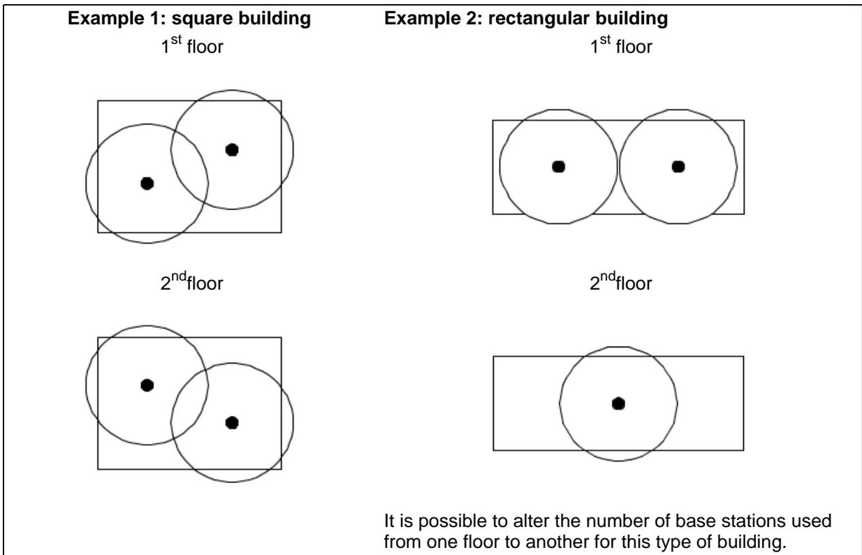
The technique used is overlapping the location of base stations from one level to another. This technique can be used for alternate floors if the coverage of a level can be achieved from an adjacent level.
