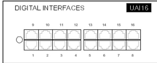
The UAI16-1 board is used to power terminals connected to the 16 interfaces remotely from an EPS48 external power supply connected to interface 1 via an external adapter cable (splitter).
