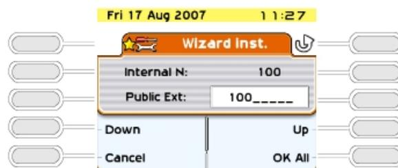
The direct number includes up to 8 digit and can be modified (the cursor is placed at the start of the field). The DDI numbers are generally the last 3 or 4 digits of your call numbers; the public operator will let you know the range of numbers that has been assigned to you.
