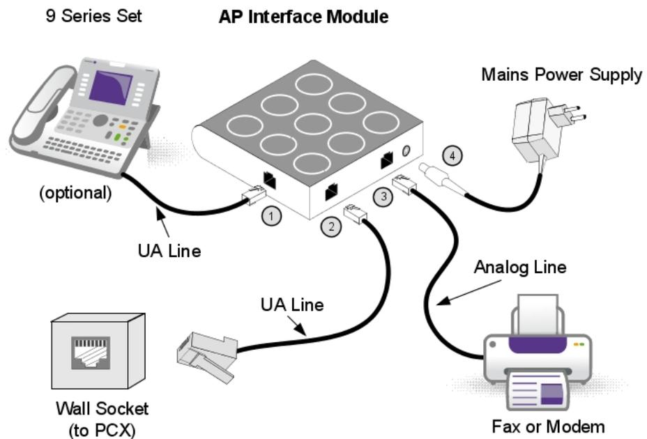
Figure 4.53: AP Interface Module Connections
