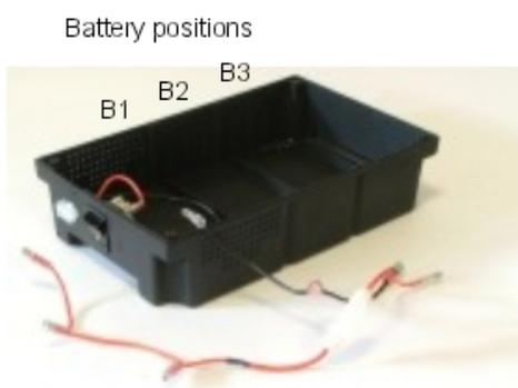
4. Connect the terminals of the batteries strictly in the order detailed below (also see the figure below).
